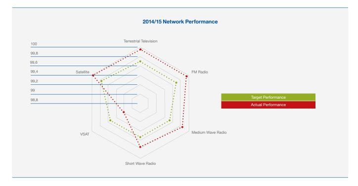
SENTECH exceeded network performance targets for Analogue Television, FM radio, MW Radio, SW radio and DTH platform services for the 2014/15 financial year. The VSAT platform performed below norm due to the unstable hub which is near its end of life (EOL). SENTECH plans to upgrade the hub during the 2015/16 financial year to improve hub performance and services reliability.
